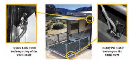
Unlatch and swing the Tailgater Kitchen (if equipped) (attached to the rear of the RV) out of the way to lower the rear ramp door. (Refer to the *Tailgater Kitchen section*)
