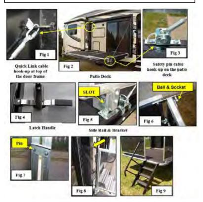
To set up the patio deck, unlatch the two keyed handles from the side of the RV ( $Fig\ 4$ ). Lower the patio deck until the cables on each side support it. Support cables are attached at the top of the door opening with a quick link ( $Fig\ 1$ ) and to the deck with a safety pin ( $Fig\ 3$ ). Patio deck is designed to be folded up with the support cables attached.
