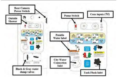
**The Uni-Doc Utility Center** is located in an exterior compartment and allows you to perform the following functions:
